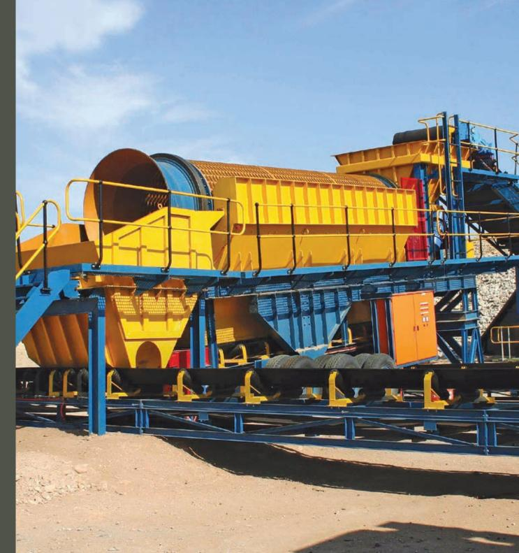
Rotary screens are employed for the scalping and size reduction of run-of-mine materials. The mobility of the rotary screens allows for in-pit screening close to the mining face, reducing the need for costly hauling of return cycles of oversize material.
