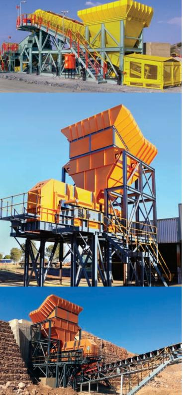
A typical plant feed bin features overhead grizzly comprising a series of equally spaced parallel bards for the scalping of oversize barren material from the run-of-mine ore. However, bin and grizzly installations of this configuration lack throughput capacity and take up much height, which necessitates the installation of a high-feed ramp to access the feed bin.
